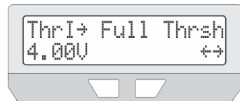
Throttle Input Voltage for Full Power
