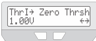
Throttle Input Voltage for Start of Power
